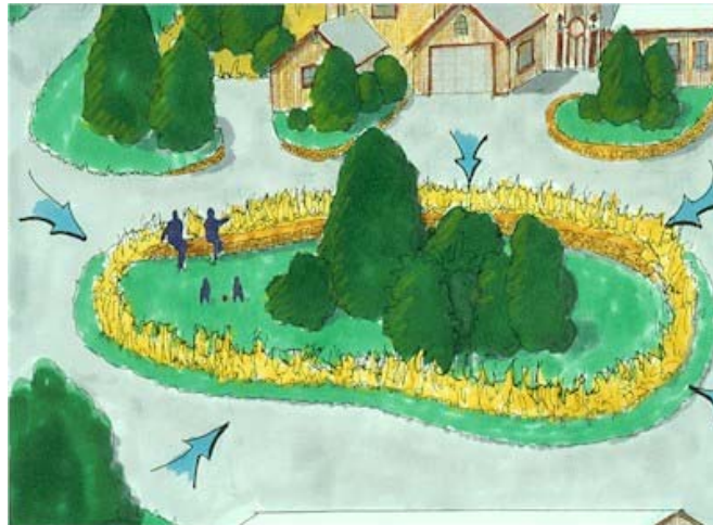
Figure 5.3-6 Natural surface depressions can temporarily store stormwater.
