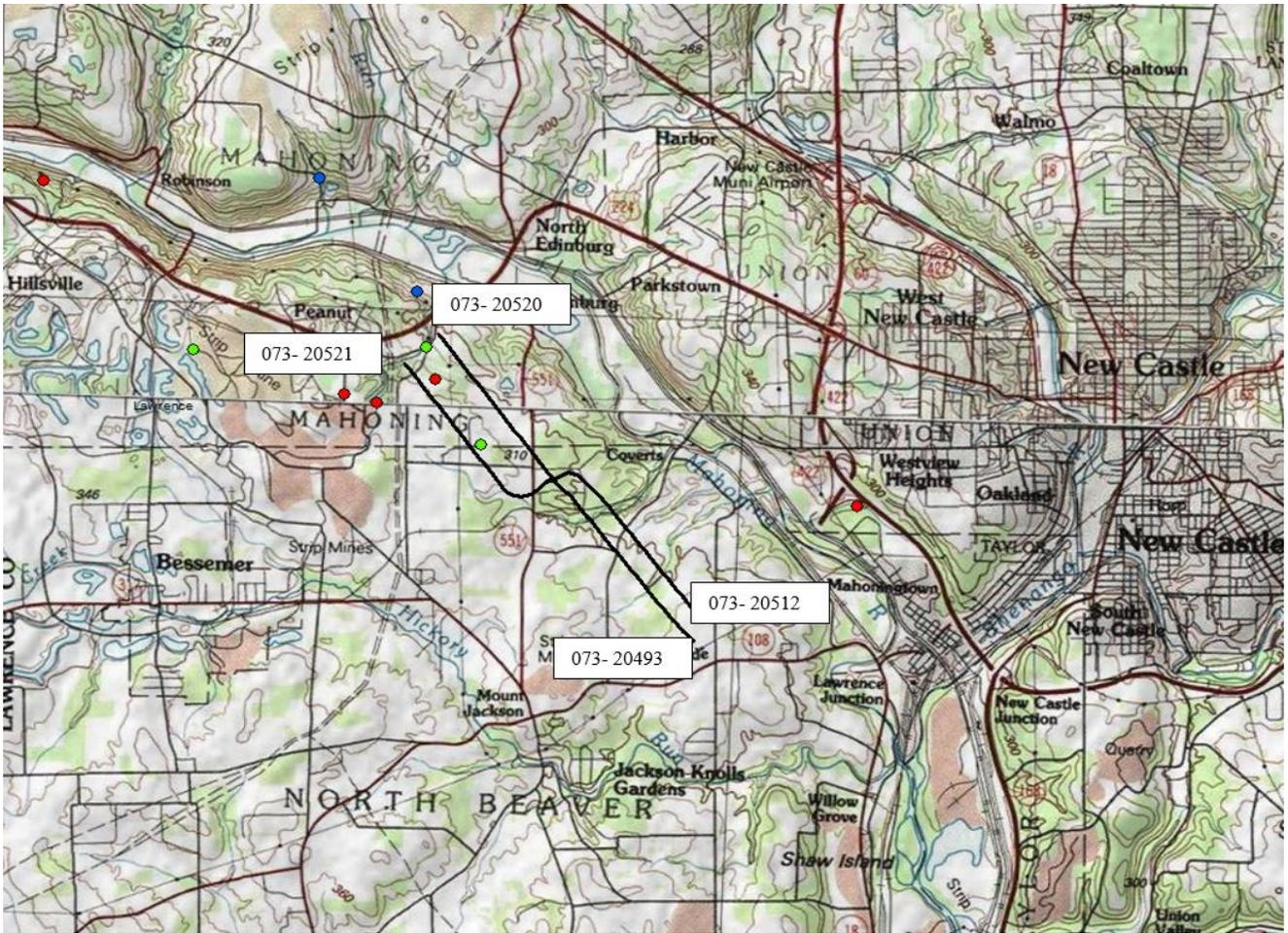
Figure 1. Location of well laterals and reported earthquake epicenters (PASeis – blue dots, OhioSeis - green dots, LCSN - red dots) in Mahoning, North Beaver and Union Townships.
